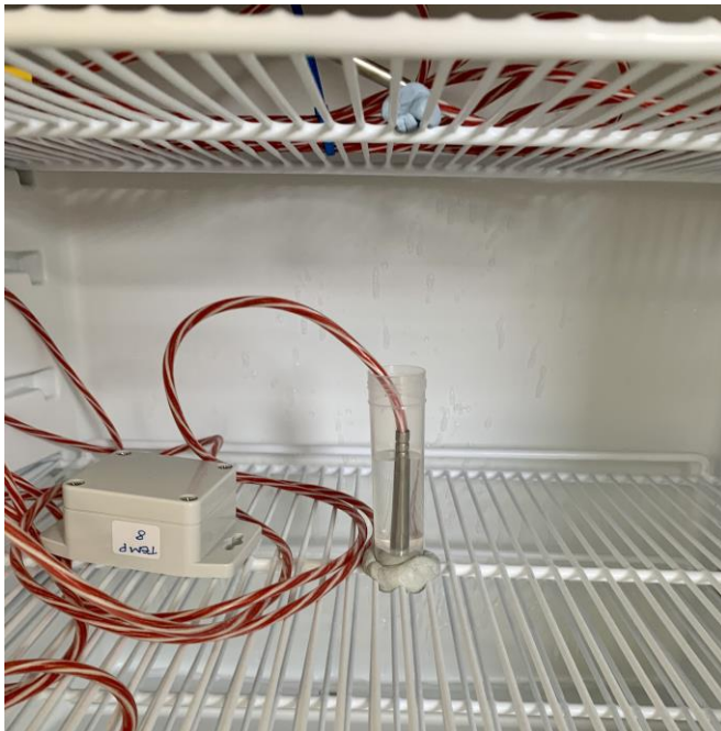
Figure 2. Sample probe was placed on the middle compartment of each unit. Central to the photo is the sample representative probe. Above this the probe in the top compartment can be seen.
